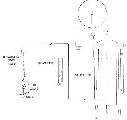
FIG. 2 Calibration Assembly Using Gasometer
