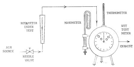
FIG. 1 Calibration Assembly Using Wet Test Meter
