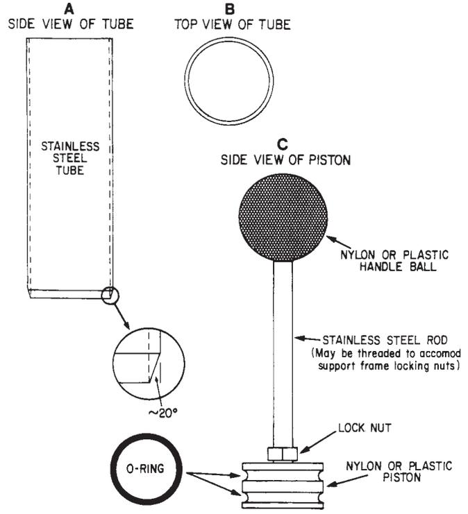
FIG. 1 Thin-Walled Piston Sampler
