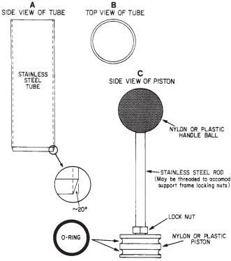
FIG. 1 Thin-Walled Piston Sampler
