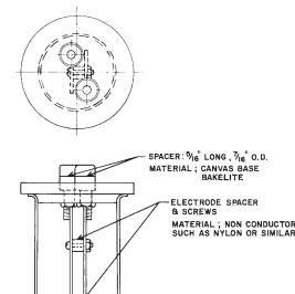
FIG. A1.2 Test Cell
