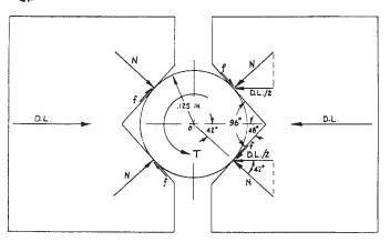
D.L. = DIRECT LOAD, LBS. T = TORQUE, IN. LBS. N = NORMAL LOAD PER FACE, LBS. u = COEFFICIENT OF FRICTION  $M_o$  = SUMMATION OF MOMENTS ABOUT POINT "O" f = FRICTION FORCE  $M_o = 0 = T - (4F \times 0.125)$ f = 2T D.L./2 = N × COS 42° N = D.L./(2 × COS 42°) N = 0.672816 D.L. u = f/N = 2T/(0.672816 × D.L.)
