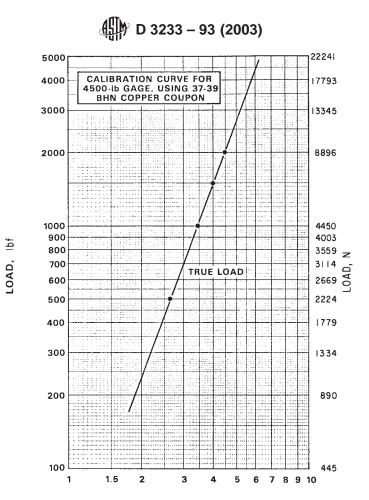
IMPRESSION DIAMETER, mm FIG. 4 Calibration Curve for 4500-lb Gage, Using 37-39 HB Copper Coupon
