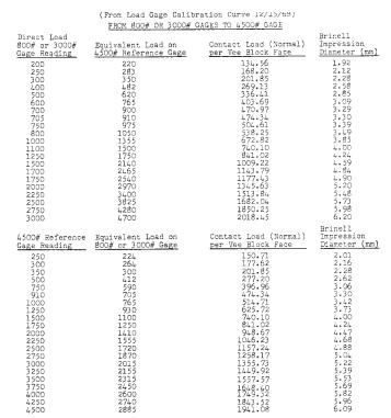
FIG. X1.2 Contact Load (Normal) per Vee Block Face and Typical Falex Load Gage Conversions
