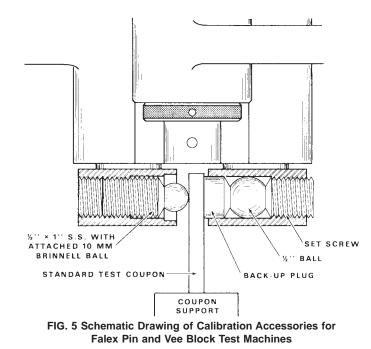
10.7 Turn off the machine and back off the load until the test coupon is free of the jaws. Advance the test coupon approximately  $\frac{3}{8}$  in. (approximately 9.5 mm). Additional indentations
