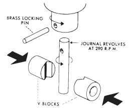
FIG. 3 Exploded View of V-Blocks and Journal Arrangement, Falex Pin and Vee Block Test Machines
