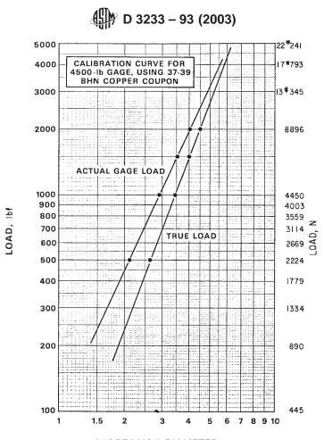
IMPRESSION DIAMETER, mm FIG. 6 Calibration Curves Used by Laboratory Reporting Data Shown in Table 1
