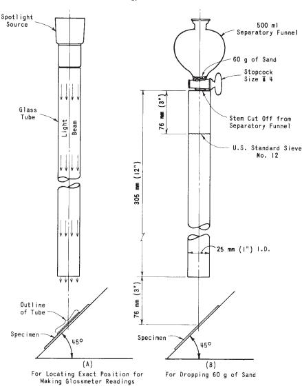
FIG. 1 Apparatus for Measuring Abrasion Resistance of Wax Coatings
