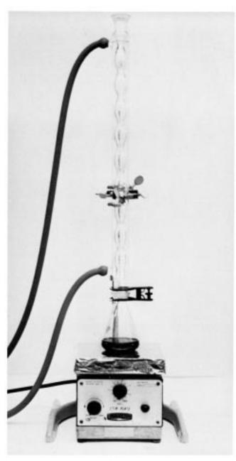
FIG. 1 Dispersing Apparatus
