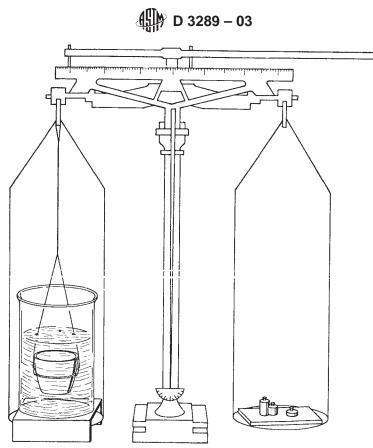
FIG. 1 Analytical Balance Equipped with Crucible Holder, Immersion Beaker, and Pan Straddle
