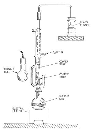
FIG. 1 Copper Stability Apparatus for Perchloroethylene
