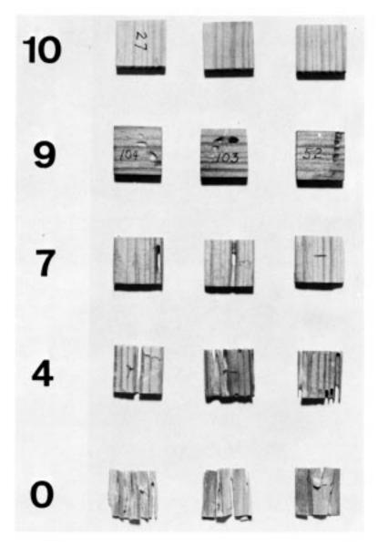
FIG. 1 Typical Ratings of Termite Attack on Test Blocks
