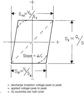
$\begin{array}{lll} V_c & = & {\rm discharge inception \ voltage \ peak \ t} \\ V_a & = & {\rm applied \ voltage \ peak \ to \ peak} \\ D_yS_y & = & Q_i \ {\rm coulombs \ per \ half \ cycle} \\ S_yS_xA & = & W \ {\rm joules \ per \ cycle} \\ A & = & {\rm area \ = \ D_xD_y} \\ AC & = & {\rm slope \ = \ C_x' - \ C_x = \ D_yS_y/D_{xa}S_x} \end{array}$
