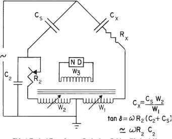
FIG. 1 Typical Transformer-Ratio-Arm Bridge (Method A)
