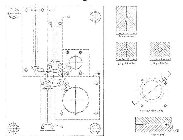
Note 1—Thermometer wells shall be 8 mm (5/16 in.) in diameter to permit use of a readily available thermometer. FIG. 1 Five-Cavity Transfer Mold for Thermosetting Plastic Test Specimens (Steam Cores Not Shown)
