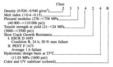
4.2 Materials used in polyethylene plastic pipe and fittings shall use a cell-type format for the identification, close characterization, and specification of material properties. The information from the format is to be used alone or in combination.
