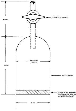
FIG. 2 Radon Scintillation Chamber
