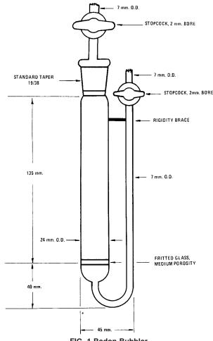
FIG. 1 Radon Bubbler
