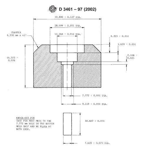
Note 1—Diameters are concentric. These two parts will be made of stainless steel. All dimensions are in millimetres. FIG. 4 Lower Half of Mold Assembly for Pressure Molding Asphalt and Pitch into a Specimen Cup
