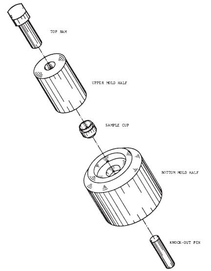
FIG. 5 Assembly of Mold for Pressure Molding Asphalt and Pitch into a Specimen Cup
