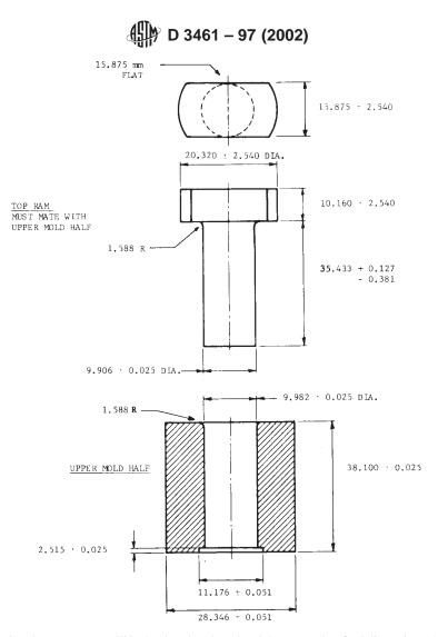
Note 1—Diameters are concentric. These two parts will be hardened tool steel and then ground to final dimensions. All dimensions are in millimetres. FIG. 3 Upper Half of Mold Assembly for Pressure Molding Asphalt and Pitch into a Specimen Cup
