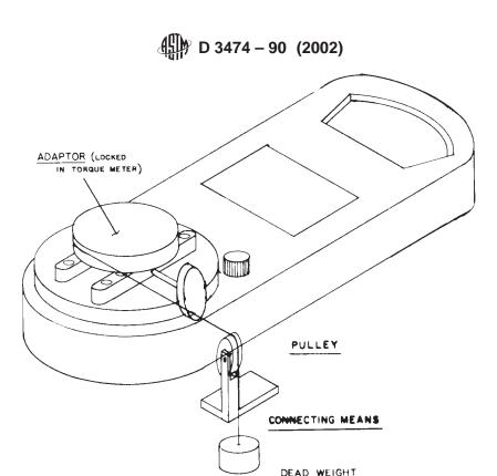
FIG. 1 Torque Meter Calibration Set Up
