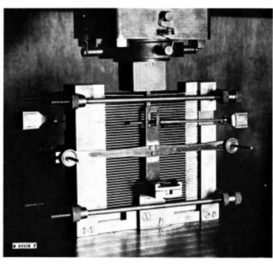
FIG. 1 Compression Test of Thin Structural Panel Supported Laterally Showing Marten's Mirror Compressometer for Measuring
