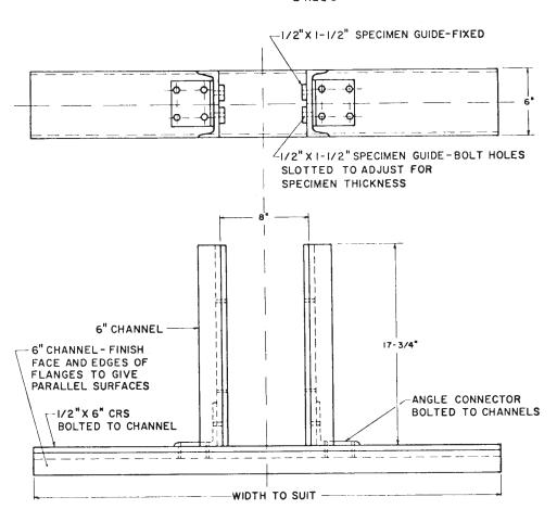
LOADING FRAME FIG. 4 Method B, Loading Hardware
