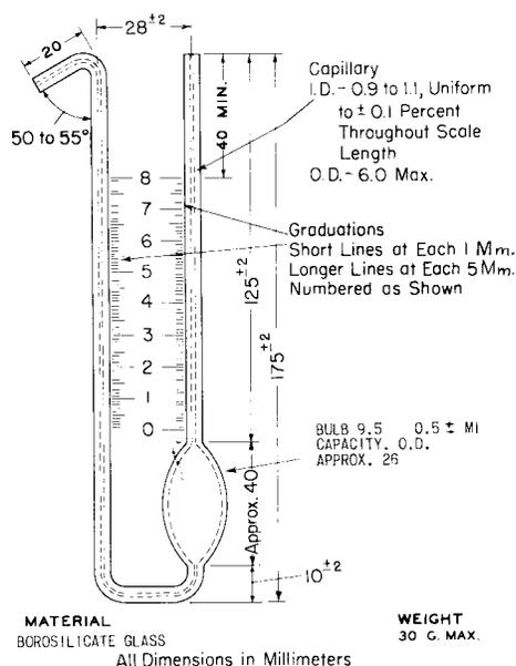
NOTE 1—The graduation lines shall extend around the entire circumference of the pycnometer at the integral numbers 0, 1, 2 cm, etc., half way around at the half divisions 0.5, 1.5, etc., and shorter lines for the intermediate subdivisions.
