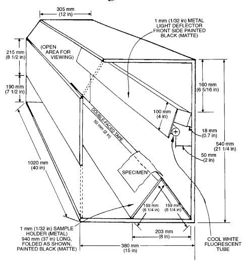
FIG. 2 Apparatus for Fabric Evaluation
