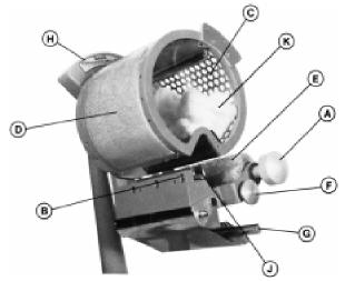
FIG. 1 Fibrosampler
