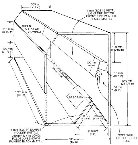
FIG. 1 Apparatus for Fabric Evaluation
