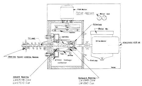
FIG. 2 Wheel Bearing Lubricant Tester (Top View)
