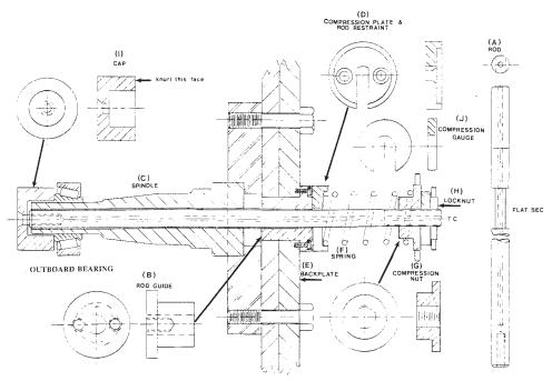
FIG. 3 Spindle and Thrust Rod Components
