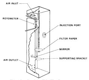
FIG. 1 Details of the Thin-Film Evaporometer
