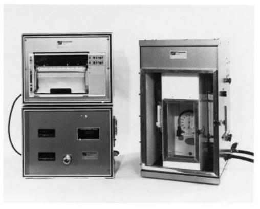
FIG. 3 Automatic Thin-Film Evaporometer
