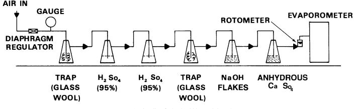
Note 1—One-litre flasks should be used throughout. FIG. 2 Diagram of Dehumidification Apparatus
