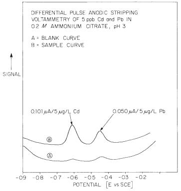
FIG. A3.1 Differential Pulse Anodic Stripping Voltammetry
