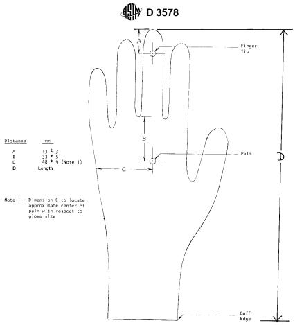
FIG. 1 Location of Thickness and Length Measurements
