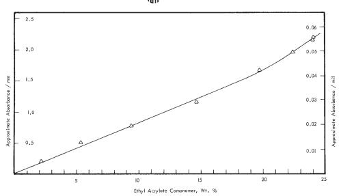
FIG. 2 Example of Typical Calibration Curve for Ethyl Acrylate Comonomer in Ethylene-Ethyl Acrylate Copolymer at 11.6 µm
