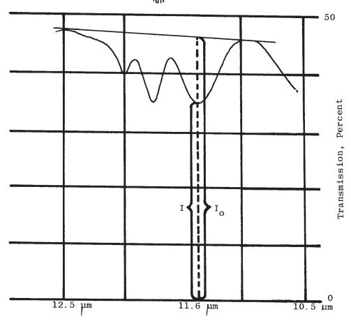
Note 1—Example illustrates baseline location, baseline wavelengths, and calculation absorbance per millimetre. Note 2—The absorbance per millimetre value, *A*, is applied to the calibration curve to obtain the concentration of ethyl acrylate comonomer.
