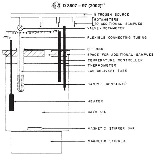
FIG. 1 Schematic of Test Apparatus
