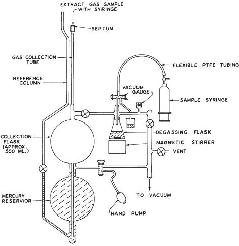
FIG. 1 Extraction of Gas from Insulating Oil
