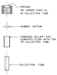
FIG. 3 Retaining Rubber Septum for Gas Collection Tube
