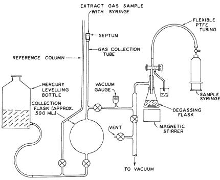
FIG. 2 Extraction of Gas from Insulating Oil
