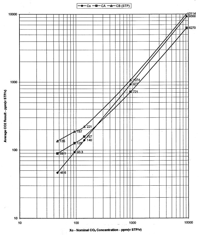
$\label{eq:Note_solution} \begin{array}{l} \text{Note } 1\text{---}\text{Co} = \text{Calculated CO}_2\\ \text{$C_A$= Average of $CO}_2$ Method A \\ \text{$C = \text{Average of $CO}_2$ Method B} \\ \text{$\textbf{FIG. 5 CO}_2$ in $Oil $--$ D 3612 A\&B Interlaboratory Test - Average Result versus Nominal Concentration} \end{array}$
