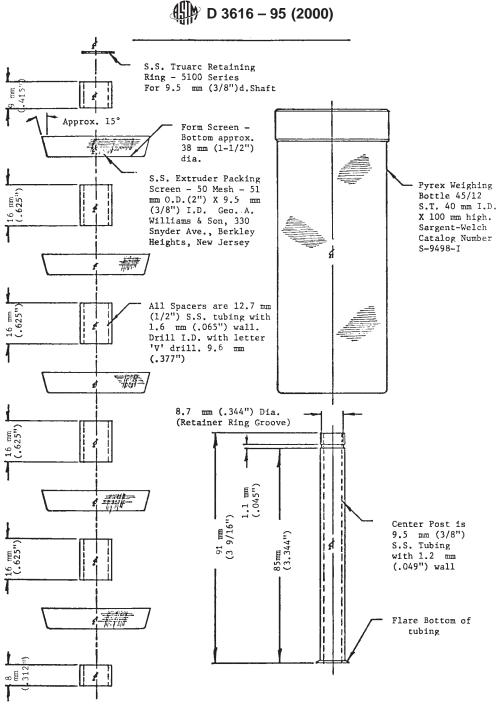
FIG. 1 Gel Test Apparatus
