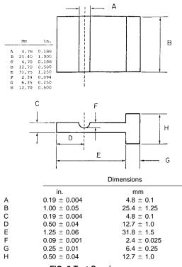
FIG. 3 Test Specimen
