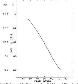
FIG. 6 Relationship Between Gap-Width and Flex Angle
