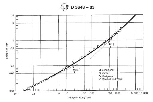
Note 1—Experimental values by several observers on monoenergetic electrons are shown. For monoenergetic electrons, the range coordinate refers to the extrapolated range. For continuous beta-ray spectra, the energy coordinate refers to the end-point energy E ..., and the range coordinate becomes the maximum range. The smooth curve represents the empirical relationship, developed by Katz and Penfeld (36).
