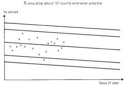
FIG. 4 Typical Counter Control Chart
