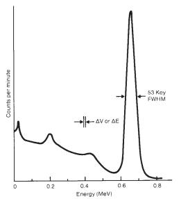
FIG. 2 Pulse Height or Energy Spectrum of Cesium-137
