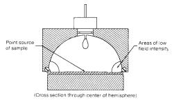
FIG. 6 Typical Chamber Geometry for Proportional Detector
