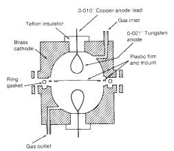
FIG. 1 The  $4\pi$ -Counting Chamber
