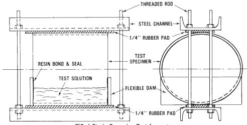
FIG. 1 Strain-Corrosion Test Apparatus
