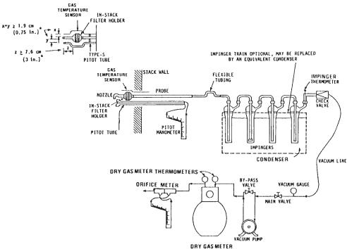
FIG. 2 (Out of Stack) Sampling Train
