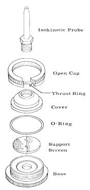
FIG. 5 Exploded Diagram for Flat, Round Filters
