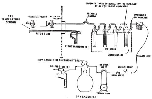
FIG. 1 Test Method A (In Stack) Sampling Train
