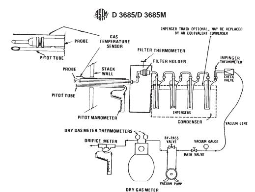
FIG. 3 Test Method A (In Stack Optional) Sampling Train
