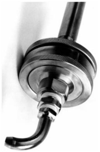
FIG. 6 Typical Holder for Flat, Round Filters
