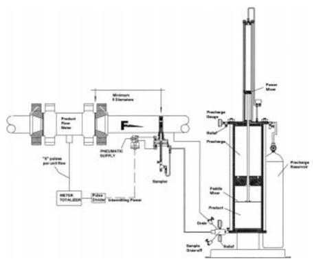
FIG. 5 Typical Sampler Using an Injection Pump
