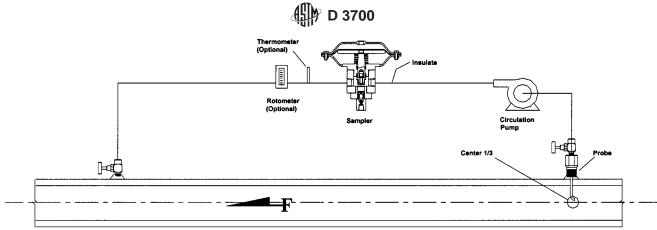
FIG. 4 Typical Sample Probe Installation for a Pump
