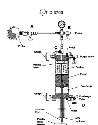
FIG. 2 Typical Sampling System
