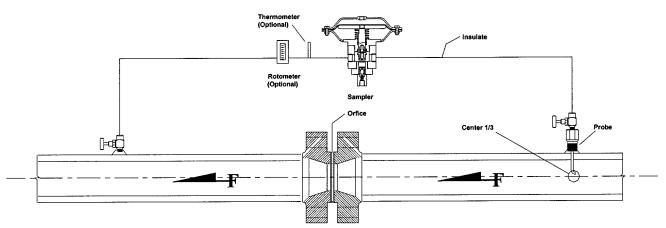
FIG. 3 Typical Sample Probe Installation on Orifice Fitting
