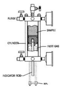
FIG. 1 Typical Floating Piston Cylinders
