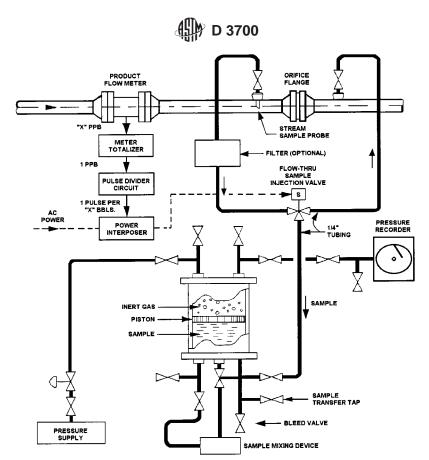
FIG. 6 Typical Automatic Proportional Sampler
