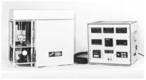
FIG. 1 The Falex Multispecimen Test Machine
