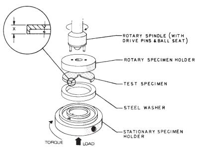
FIG. 2 Thrust Washer Test Specimen Arrangement
