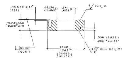
FIG. 4 Stationary Steel Washer Specimen
