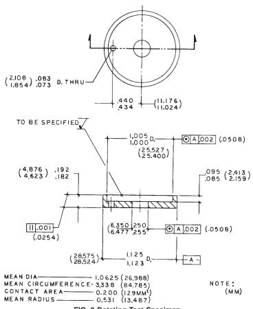
FIG. 3 Rotating Test Specimen
