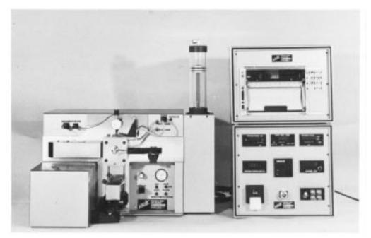
FIG. 1 Falex Block on Ring Test Machine
