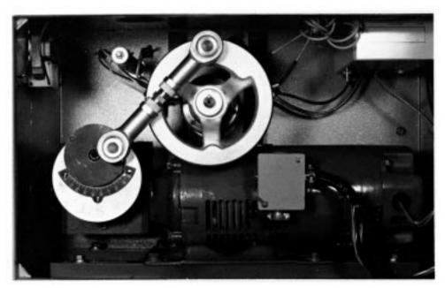
FIG. 2 Falex Oscillating Drive Assembly
