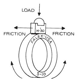
FIG. A1.1 Schematic Drawing of Ring & Block Specimens in Oscillating Motion
