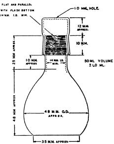
FIG. 2 Pycnometer for Determining Relative Density of Petroleum Sulfonates
