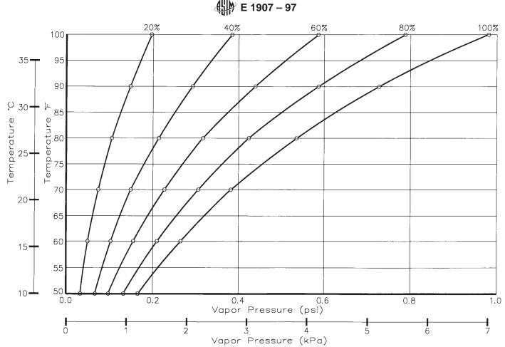
FIG. X1.1 Vapor Pressure of Moisture in Air at Different Temperatures and Relative Humidities. (Source: Ashok Kakade)
