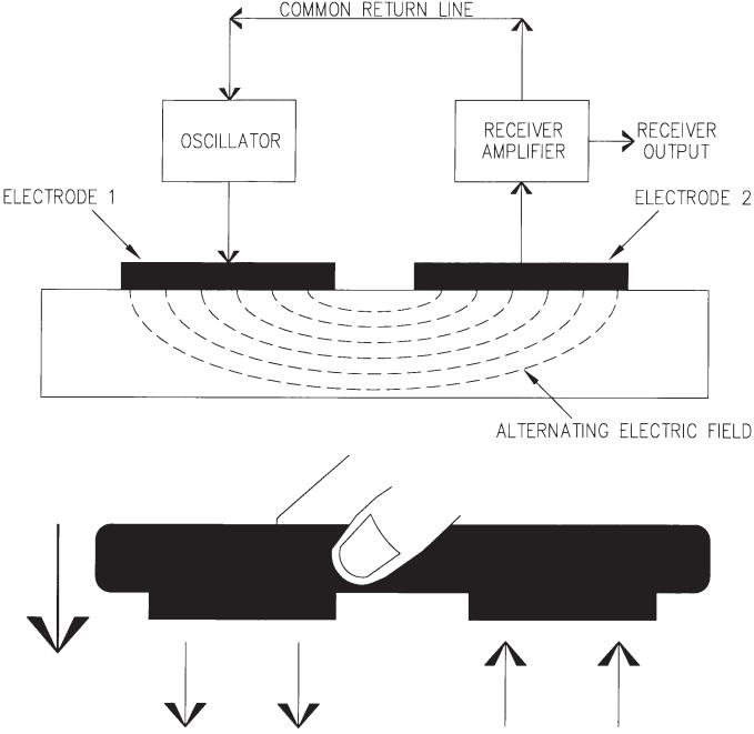
FIG. 1 Basic Schematic of Electrical Impedance Moisture Meter
