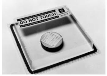
FIG. 2 Anhydrous Calcium Chloride Test
