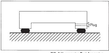
FIG. 3 Hygrometer Test Apparatus
