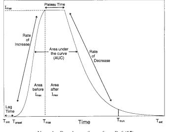
Note 1—Based on a figure from Ref (15). FIG. 1 Representative Time-Intensity Curve with Selected Parameters Labeled
