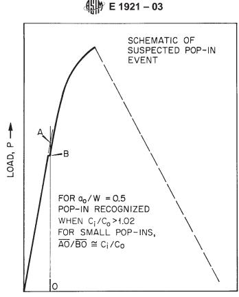
DISPLACEMENT, V → FIG. 6 Schematic of Pop-in Magnitude Evaluation
