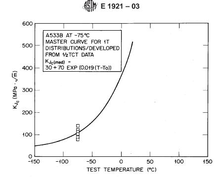
NOTE 1-Toughness data are converted to 1T equivalence. FIG. X2.1 Master Curve for 1T Specimens Based on 1/2T Data Tabulated in Step X2.2
