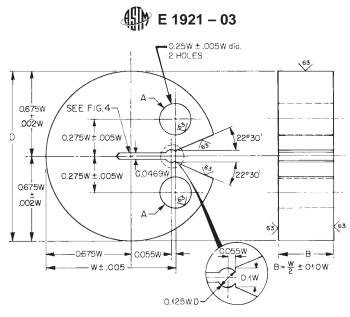
Note 1—A surfaces shall be perpendicular and parallel as applicable to within 0.002W TIR.
