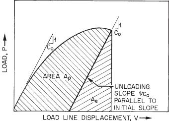
FIG. 5 Definition of the Plastic Area for  $J_p$  Calculations
