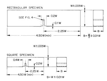
Note 1—All surfaces shall be perpendicular and parallel within 0.001W TIR; surface finish 64v. Note 2—Crack starter notch shall be perpendicular to specimen surfaces to within $\pm$  2°. **FIG. 3 Recommended Bend Bar Specimen Design**
