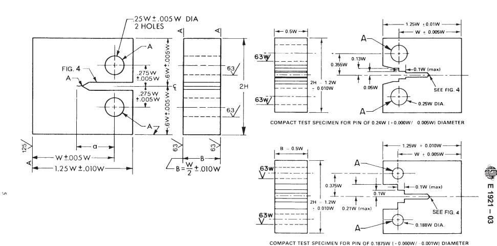
NOTE 1—"A" surfaces shall be perpendicular and parallel as applicable to within 0.002W TIR.
