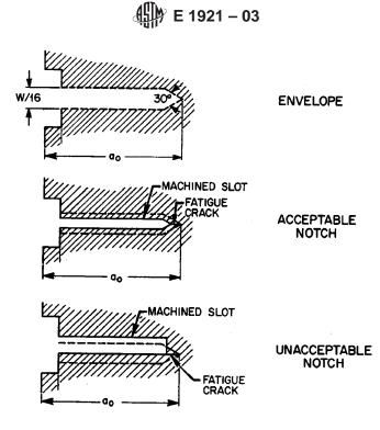
Note 1-Notch width need not be less than 1.6mm (1/16 in.) but not exceed W/16.
