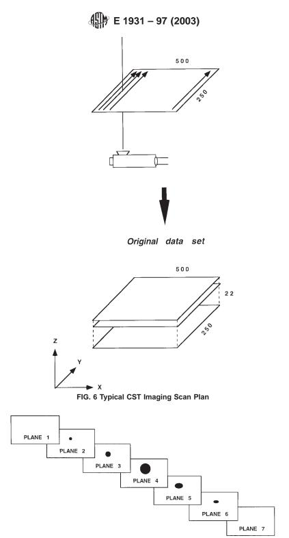
FIG. 7 Simulated CST Image Display of a Homogenous Examination Object Containing a Void
