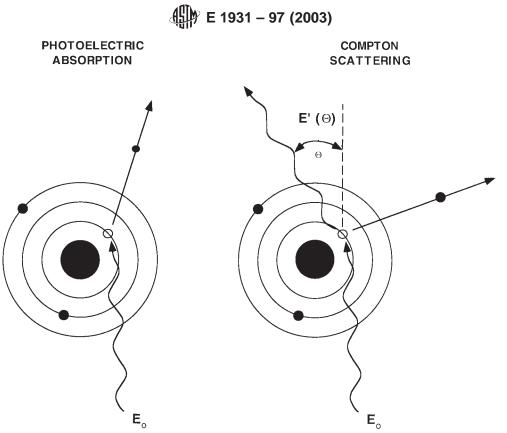
FIG. 2 Principals of Photoelectric Absorption and Compton Scattering
