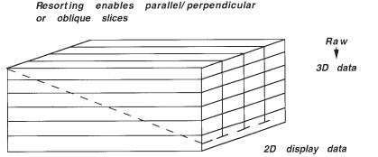
FIG. 11 Tomographic Slice Images May be Generated at Any Angle With Respect to the Original Slice Images
