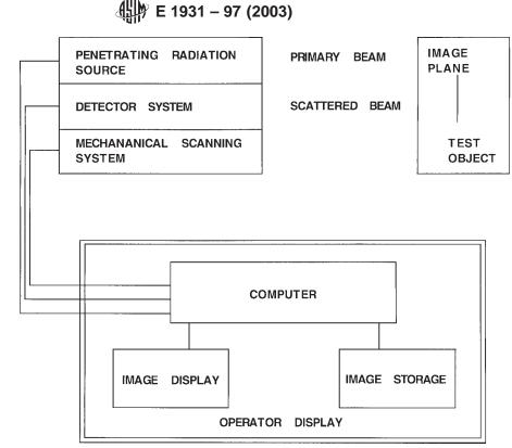
FIG. 8 Typical CST System Block Diagram
