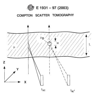
FIG. 5 Schematic Representation of the Compton Scatter Tomography Technique
