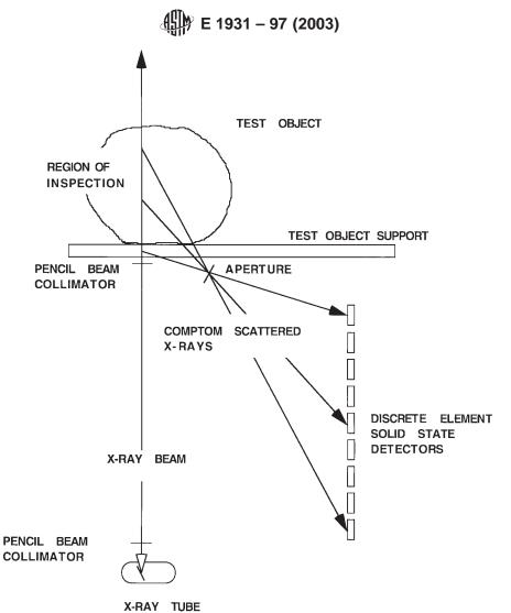
FIG. 9 General Arrangement of X-Ray Source, Detector Array and Examination Object for a Simultaneous Multi-Plane Compton Tomographic Imaging System
