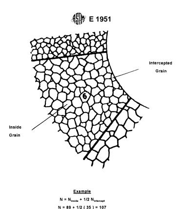
Note 1—A schematic diagram illustrating the counting of the number of grains per sector.
