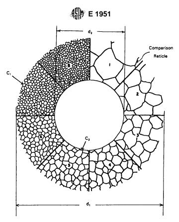
Note 1—A schematic diagram illustrating the measurements described in 5.7.4.2 and 5.7.4.5.
