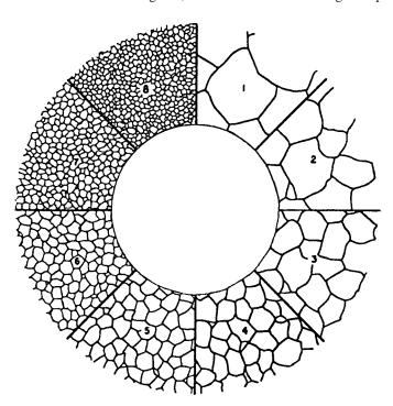
Note 1—A schematic diagram representing a grain size comparison reticle. FIG. 4 Representation of Grain Size Comparison Reticle
