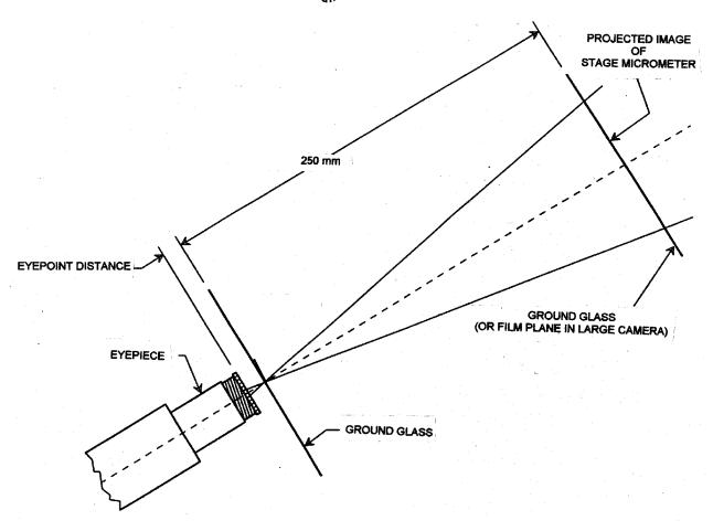
Note 1—A schematic diagram illustrating the procedure used to determine the magnification observed through the microscope eyepieces.
