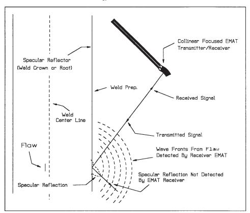
FIG. 4 The Diffraction Technique
