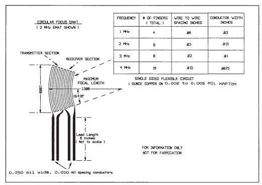
FIG. 5 Design Parameters for Typical Focused EMAT Coil
