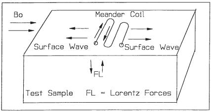
FIG. 1 Typical EMAT Configuration for Rayleigh Wave Generation
