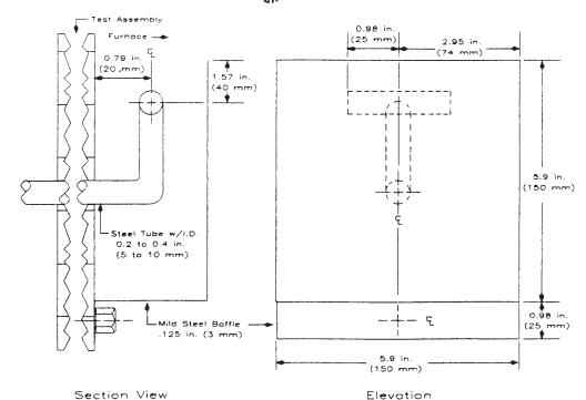
FIG. 3 "T" Shaped Pressure Sensing Probe
