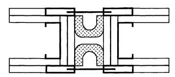
Typical Symmetrical Wall-to-Wall Joint System
