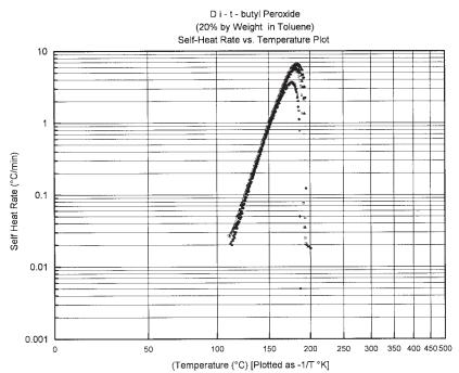
FIG. X1.1 Di-t-Butyl Peroxide (20 Weight Percent in Toluene) Self-Heat Rate vs. Temperature Plot
