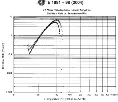
FIG. X1.3 2 to 1 Molar Ratio—Methanol to Acetic Anhydride Self-Heat Rate vs. Temperature Plot
