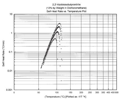
FIG. X1.2 2,2'-Azobisisobutyronitrile (12 Weight Percent in Dichloromethane) Self-Heat Rate vs. Temperature Plot
