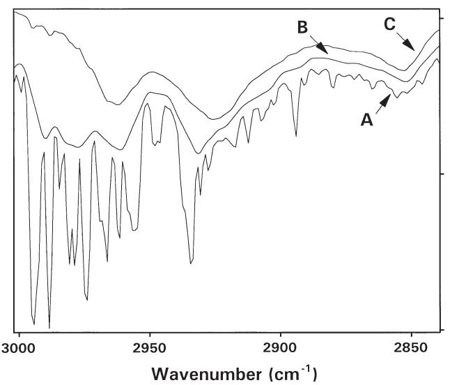
FIG. 2 Single-beam OP/FT-IR spectra collected at 2-cm<sup>-1</sup> resolution representing: (A) a field spectrum acquired over a 200-m path; (B) a synthetic background spectrum; and (C) a short path background spectrum. The positions of the spectra are offset slightly on the ordinate for clarity.
