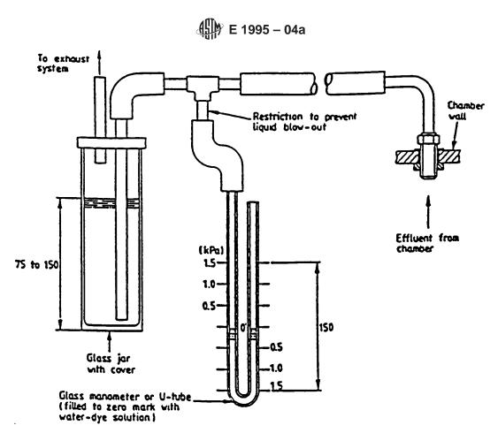
Note 1—All dimensions in this figure are given in mm unless stated otherwise. FIG. 3 Typical Chamber Pressure Relief Manometer
