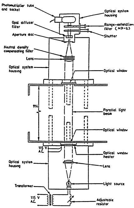
Note 1—The dimensions in this figure are given in mm unless stated otherwise. FIG. 10 Photometric System
