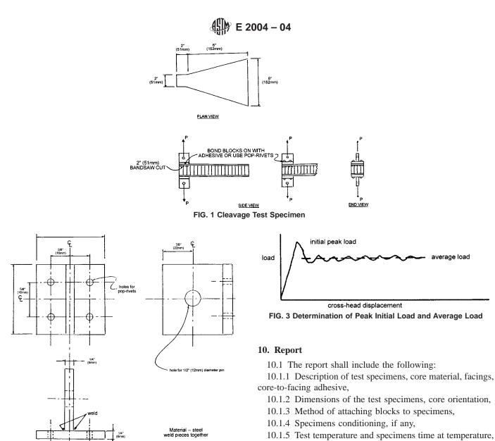
FIG. 2 Loading Blocks for Cleavage Test Specimen
