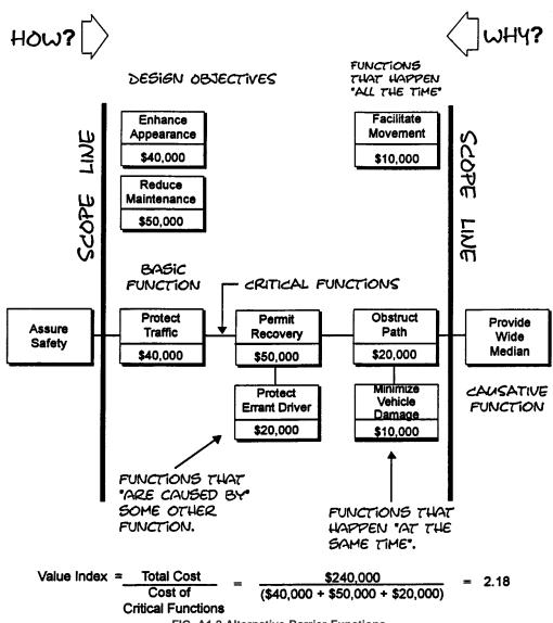
FIG. A1.2 Alternative Barrier Functions
