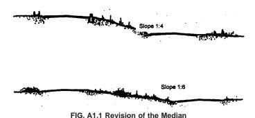
A1.3.2 Plant low-level bushes that would obstruct the path of an errant vehicle, slowing it down and protecting the driver.
