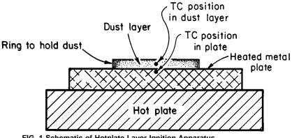
FIG. 1 Schematic of Hotplate Layer Ignition Apparatus
