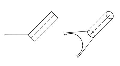
FIG. 3 Scoop Used to Remove Spillage
