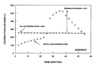
FIG. X3.1 Examples of Hotplate Layer Ignition Test Data
