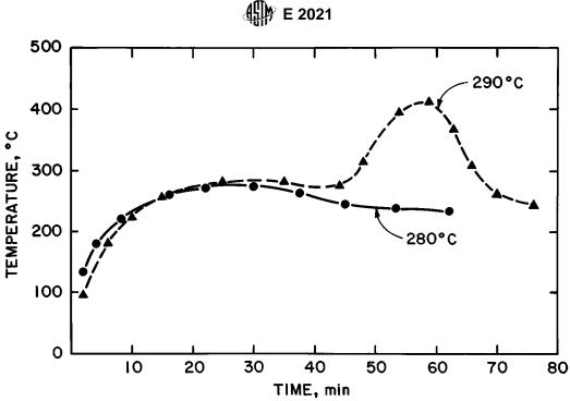
FIG. 4 Test Data Showing Nonignition at Set Temperature of 280°C and Ignition at Set Temperature of 290°C
