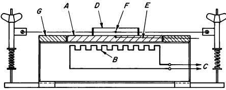
FIG. X2.1 Hot-Surface Layer Ignition Apparatus
