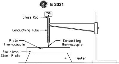
FIG. X2.3 Measurement of Surface Temperature Distribution
